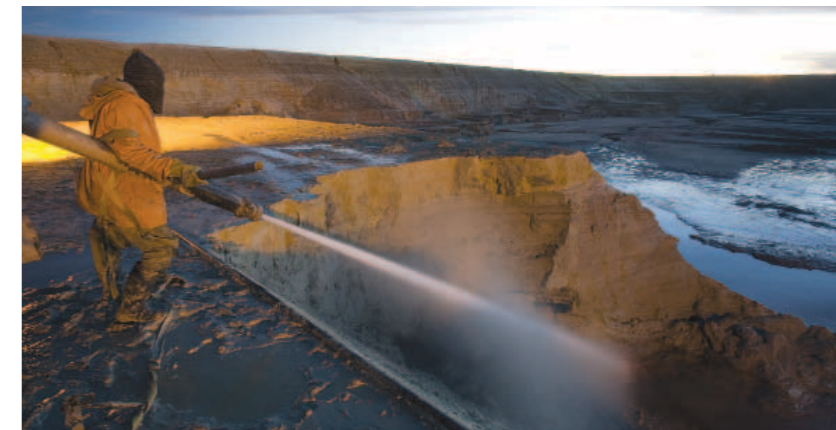
Hydraulic reclamation of mine residues is one of the services offered by the Tailings Operations division.
