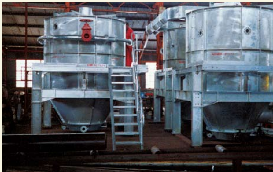
A surface installation of the Skelton & Plummer High Rate Clarifier.
