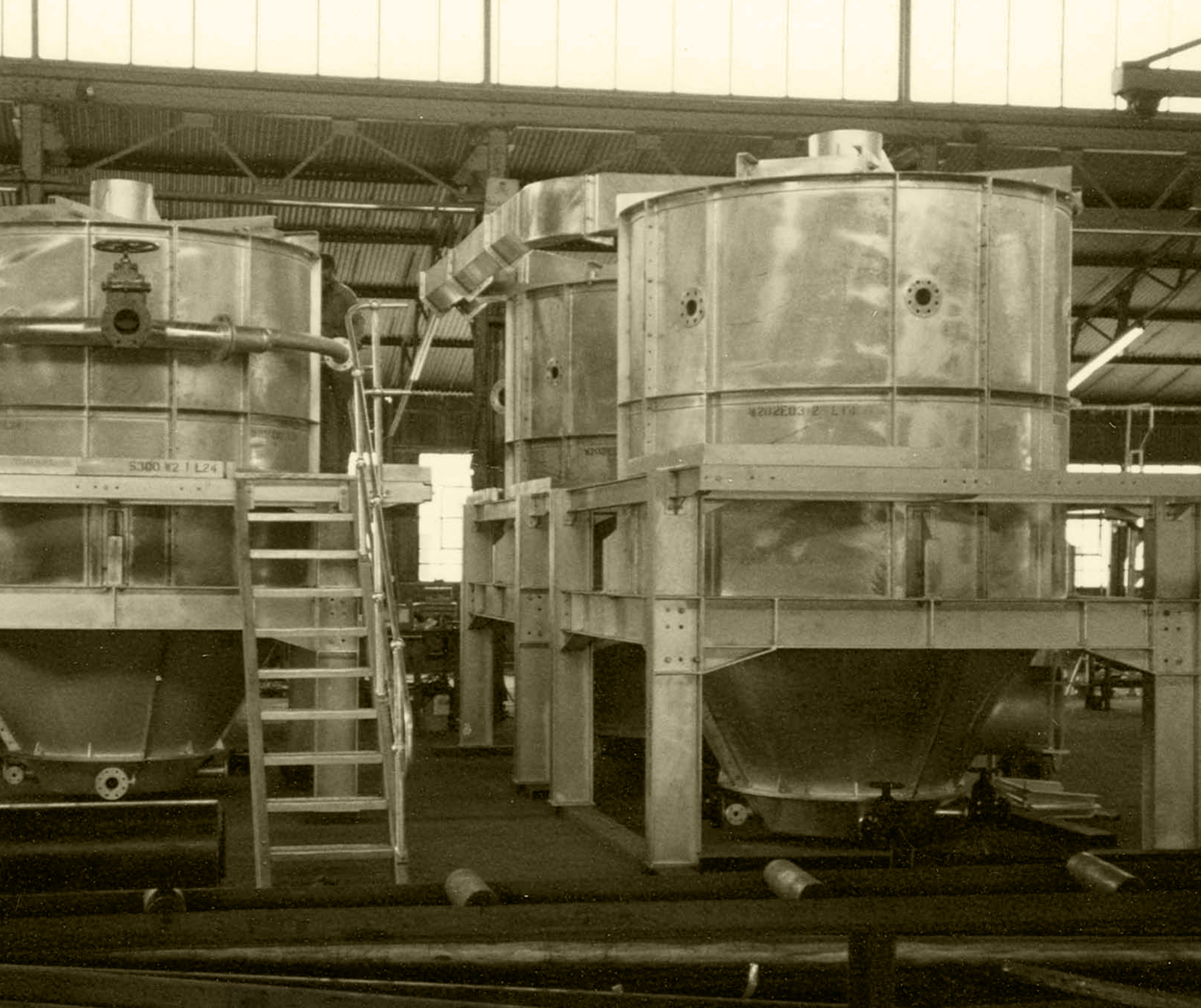
The Skelton & Plummer high-rate clarifier (S&P HRC).
